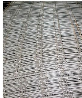
The new product is available in two different styles of mesh produced using two different alloys. One product is 6X6 D2.9/D2.9 (gage) that would be assembled in 6-foot x 12-foot mats. The other product is 4X4 D4/D4 (gage) available as 6-foot x 12-foot mats. These sizes are the most popular in carbon mesh. All stainless wire mesh is branded with "SALIT" so buyers know that the wire mesh they are using is from a source in the Salit Group of Companies.
