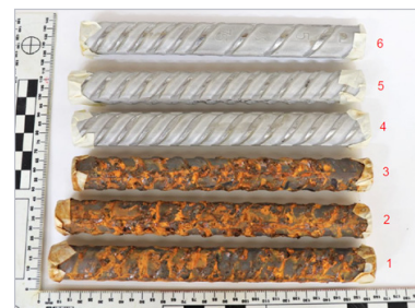
Photo of samples after 96 hours of salt spray exposure
